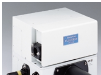
SIM Scanner Second scanner dedicated for laser light stimulation, synchronized to the FV1000 main scanner for simultaneous laser stimulation and confocal image acquisition. Independent fiber optic laser introduction port. Dichromatic mirror within motorized optical port of the scan unit required for introduction of laser into main scanner.
