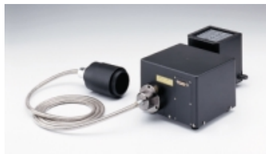
Transmitted light detection module External transmitted light photomultiplier detector and 100W Halogen conventional illumination, integrated for both laser scanning and conventional transmitted light Nomarski DIC observation. Motorized exchange between transmitted light illumination and laser detection. Simultaneous multi-channel confocal fluorescence image and transmitted DIC acquisition enabled.
